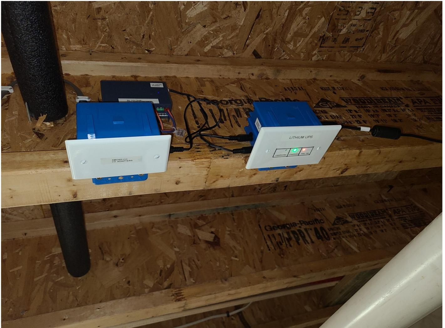
I also desoldered the 3 indicator LED's on the board (red on/off, red charging, green fully charged), and added flying-lead LED's, which I then glued to the blank plate where I had drilled 3 holes for the lights to shine through.
