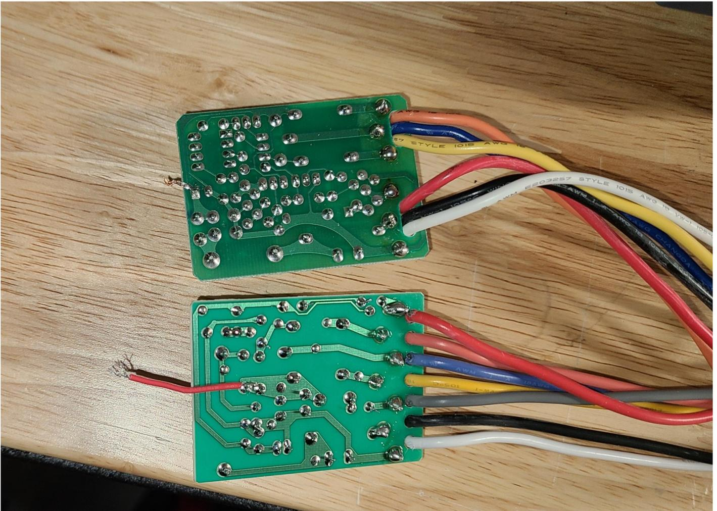
Top board is the CO alarm, bottom board is smoke alarm. The CO alarm looks a bit more complicated, because it is. The smoke alarm signal is a simple high/low signal on the RED wire, with some filtering to keep the CO signal from triggering it, so it is pretty straightforward. But the CO alarm has to run its signal on the same wire, so to differentiate between CO and smoke, the CO alarm is actually sending serial data, which requires a chip to decode.
