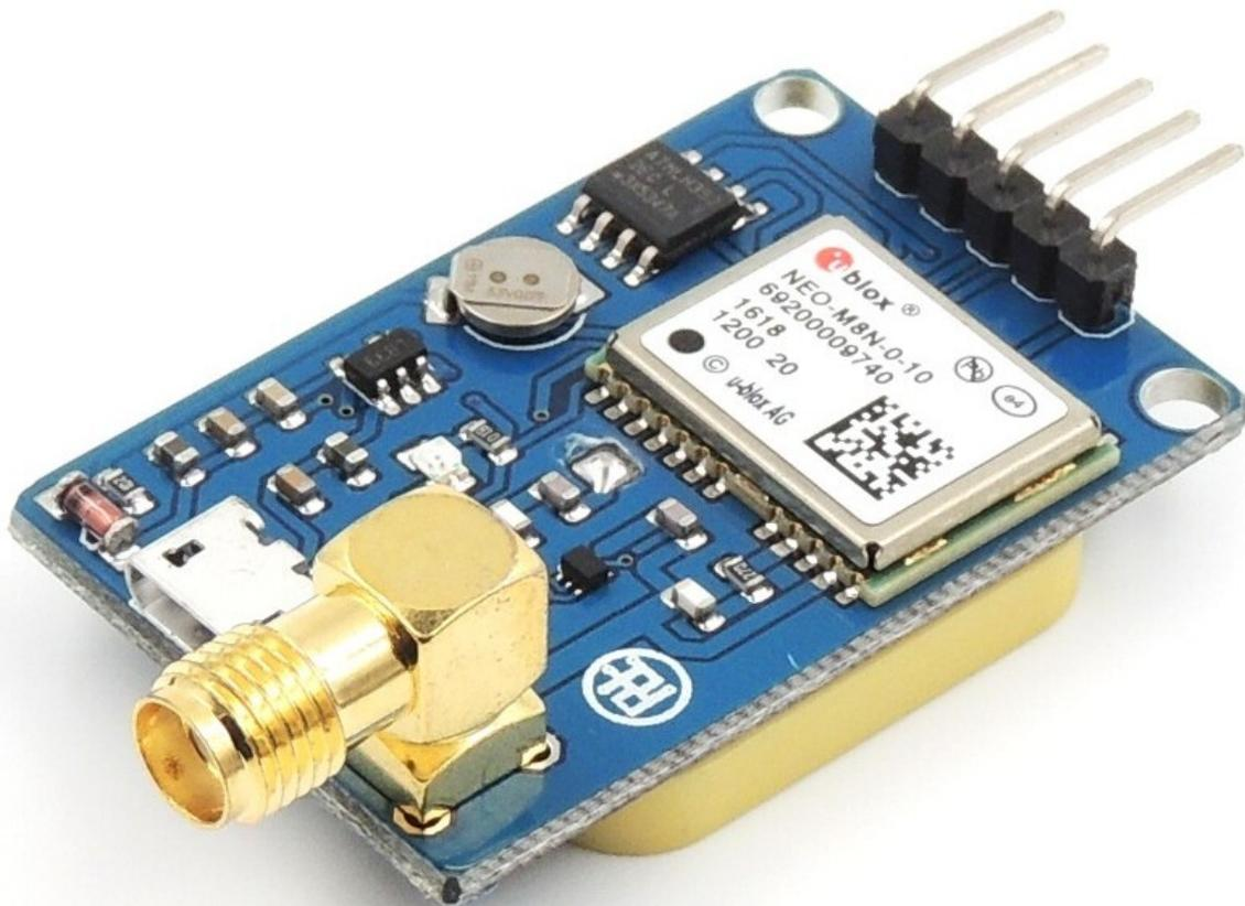
Things of note: GPIO header, USB, included antenna module, and external antenna port:
