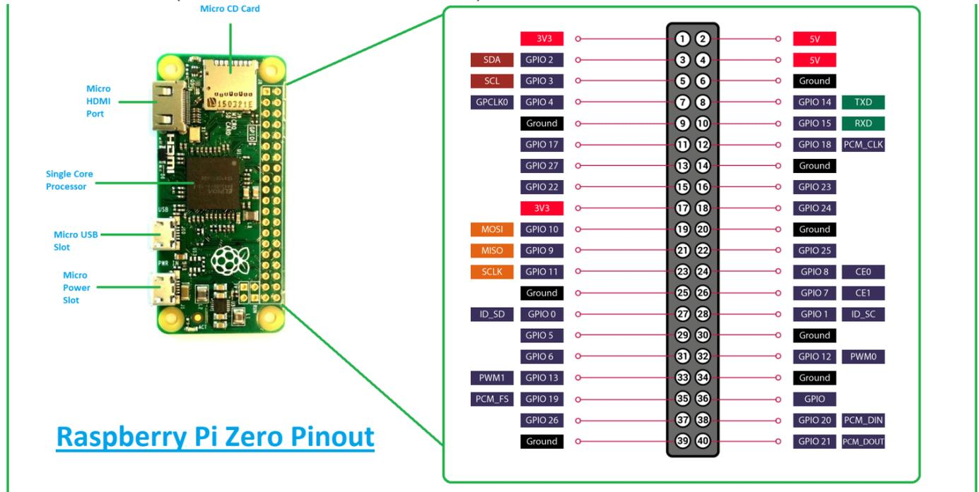
Note that all the required pins on the Pi header are sequential. Most GPS modules with headers are pin-compatible with the Pi, however some swap the positions of the TX and RX pins (The 'TX' of the GPS module must go to the 'RX' pin on the header, and vice-versa.) If the GPS is not detected when you plug it into the header, try extending the header with jumper wires and crossing over the TX/RX pins.
